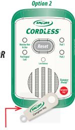
When using "Reset Button OFF" Place the Caregiver Key<sup>™</sup> over the red dot to reset the monitor.
